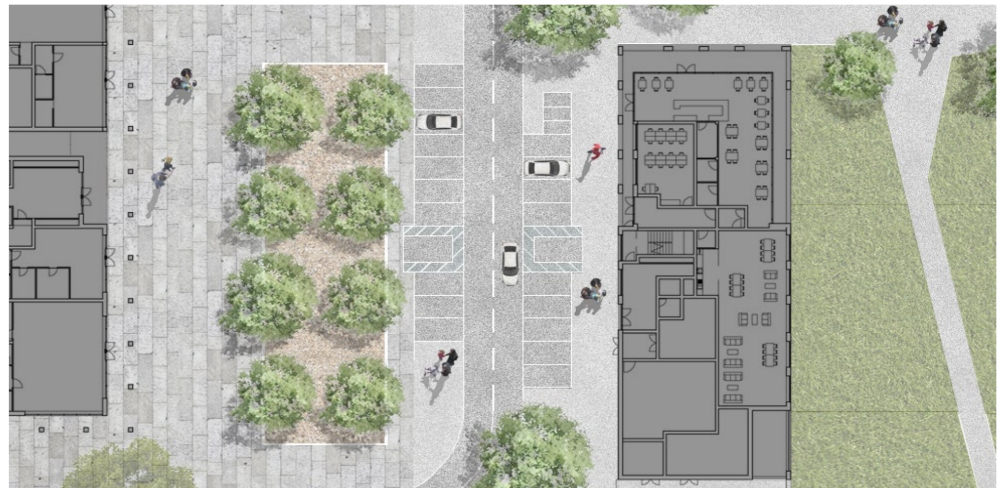
Landscape Diagram: A shared surface extends across roads to create a pedestrian friendly public space.
